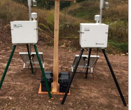
Dust-monitoring equipment used for the Short Term Ambient Air Quality Monitoring.
