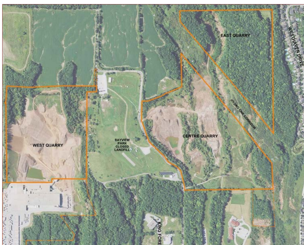
This map illustrates Meridian Brick's Aldershot Quarry complex in Burlington. Orange boundaries indicate the three elements of the quarry: Aldershot West, Aldershot Centre and Aldershot East. Currently, Aldershot West and Aldershot Centre are almost depleted, and most of the remaining Queenston shale in the quarry complex is located in Aldershot East.
