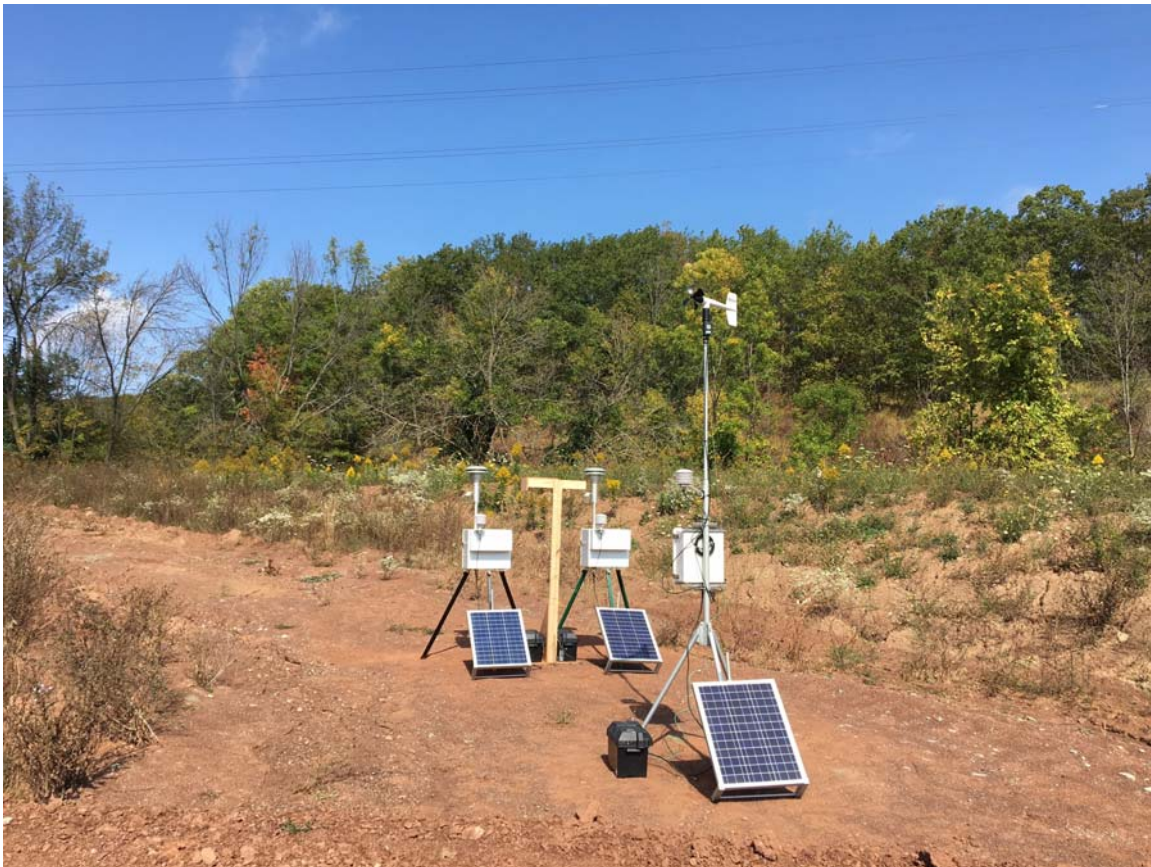
Figure 1.2.3. Ambient Air Quality Monitoring Station STN1 and MET Tower
